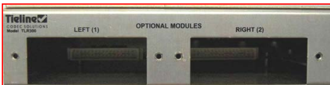
Figure 6: Module Slots on a Rack Unit Codec
