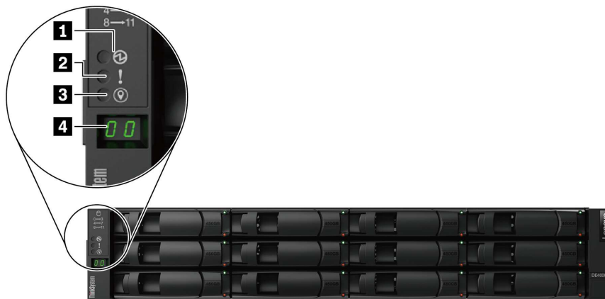
Figure 50. LEDs on the operator display panel
