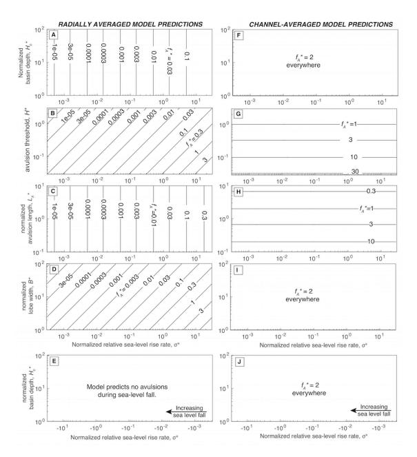
**Fig. 2.S2.** Normalized avulsion frequency predictions according to the radially averaged model (A-E) and channel-averaged model (F-J), with systematic variation of basin depth, avulsion threshold, avulsion length, and lobe width. Other model parameters were set to constant values typical of large lowland deltas ( $H^*$  =
