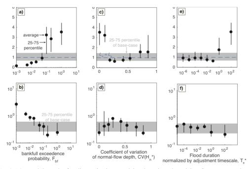
**Fig. 3.14:** Model results for dimensionless avulsion length and avulsion frequency under changing bankfull exceedance probabilities (a-b), coefficients of variation of normal-flow depth (c-d), and normalized flood durations (e-f). Black circles show average and 25-75 percentile range of avulsion location and frequency. Gray shaded regions denote the 25-75 percentile range for a stable climate in the base-case simulation. Blue dashed line indicates where  $L_A = L_b$ .
