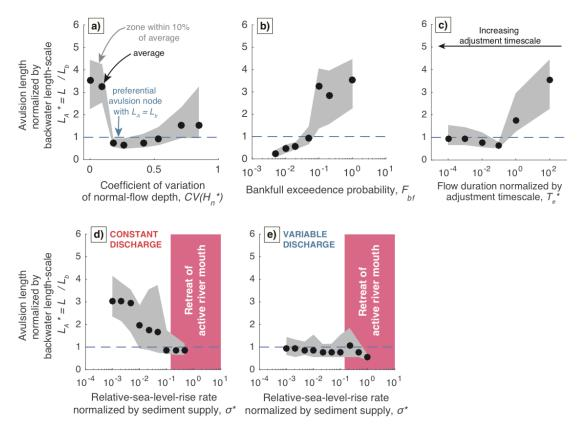
**Figure 1.3:** Model results for avulsion length with changing flow variability parameters: CV (a),  $F_{bf}$  (b), and  $T_e^*(c)$ , as well as variation of relative-sea-level-rise rate  $\sigma^*$  under constant discharge (d) and variable discharge (e). Black circles show avulsion locations averaged over cycles not influenced by
