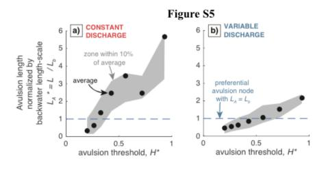
**Figure 1.S6:** Model results for avulsion length with changing avulsion threshold  $H^*$  under constant discharge (a) and variable discharge (b). Each black circle shows the avulsion locations averaged over cycles not influenced by the initial conditions (cycles 5-13), and the gray shaded areas denote the average reach within 10% of the avulsion threshold at times of avulsion. For all model runs,  $Fr_{n,bf} = 0.17$ ,  $\tau_{n,bf}^* = 1$ ,  $C_f = 0.005$ , and  $H_b^* = 2$ .
