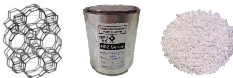
Figure 2.6. ZSM-5 catalysts for deactivation (pyrolysis) and regeneration (ozonation) studies.
