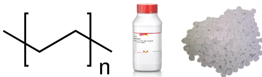
Figure 2.5. Polyethylene used as plastic feedstock for pyrolysis experiments.
