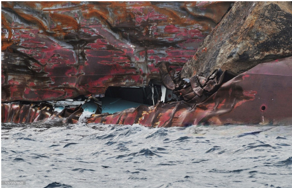
Figure 2.3: Costa concordia grounding damage - From [22]
