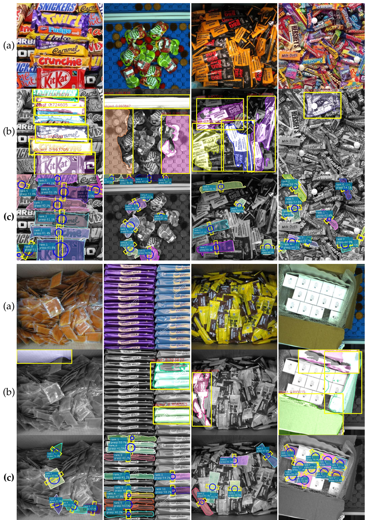
Figure 4.26: Comparative instance segment proposals after training on Mikado. From top to bottom: input (a); results using a proposal-based approach [45] (b); using the proposed approach (c). On (b), the rectangles are the detected box proposals. On (c), the rectangles and circles represent instance-centered parallel-jaw and suction-cup grasps respectively.
