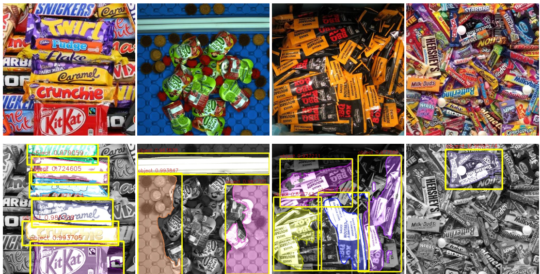
(c) As a result, a box proposal-based segmentation approach [45] gives poor results on dense piles of sachets. First row: input; second row: best-scored detected box proposals (yellow rectangles) and corresponding binary segmentations (colored areas) after training on our synthetic training data. Best viewed in color
