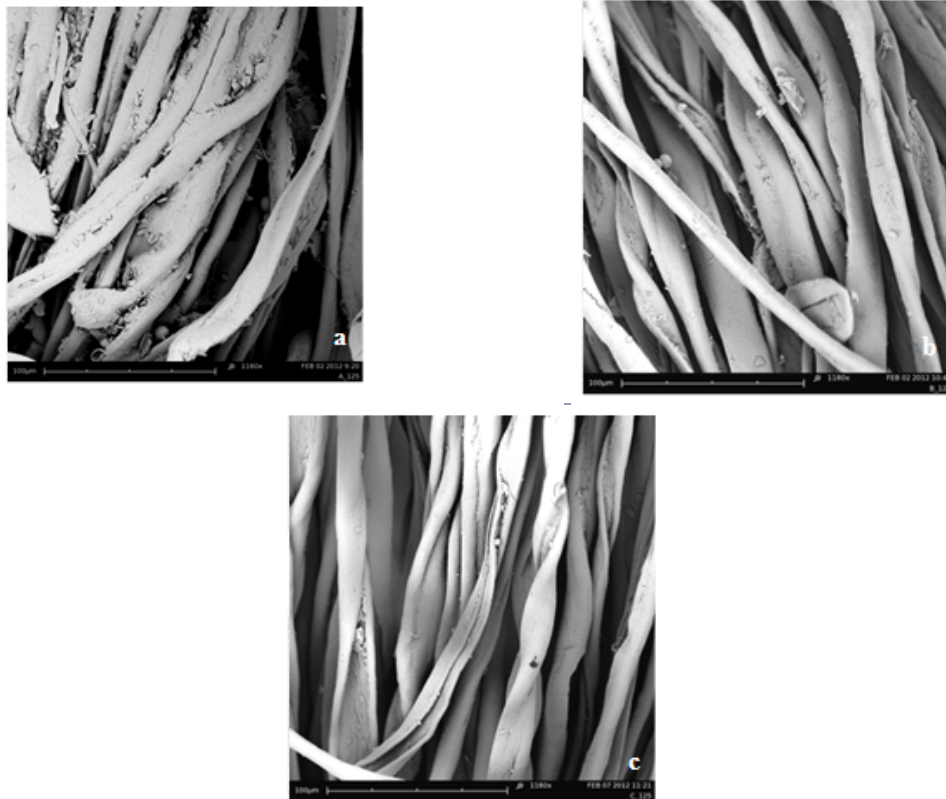
Figure 1: SEM micrographs of cotton fabrics after 125 abrasion cycles (a) Cotton 1. (b) Cotton 2. (c) Cotton 3
