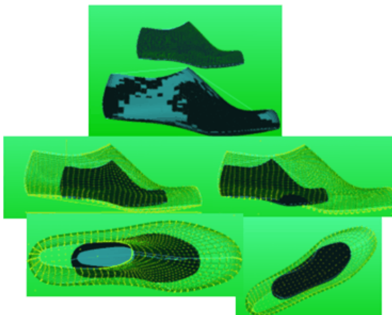
Figure 6: The results for comparing LAST1 with LAST2 after modifying the parameters of the last 1 with parameters of the last2
