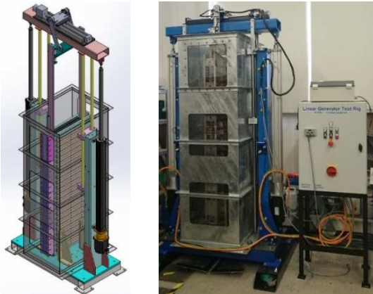
Fig. 23. Left: CAD detail of 5 kW C-Gen machine and test rig. Right: Fabricated test rig installed at the University of Edinburgh.
