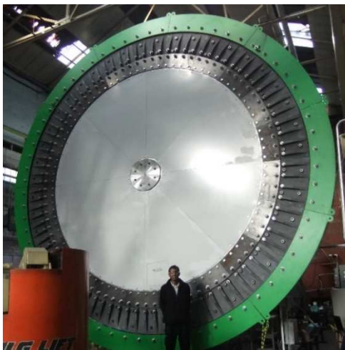
Fig. 2. 1 MW axial flux multi-stage rotary machine
