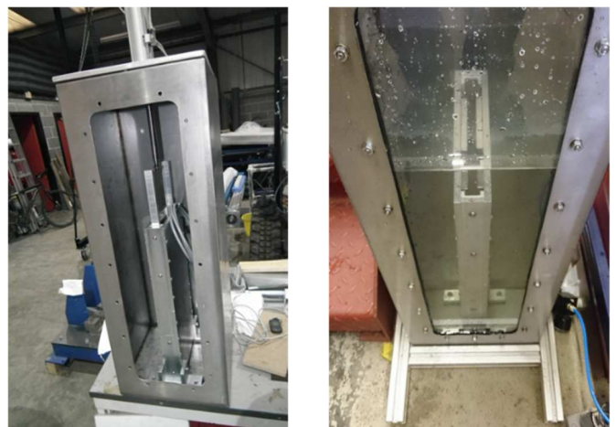
Fig. 18. Linear test rig with a miniature PM machine.
