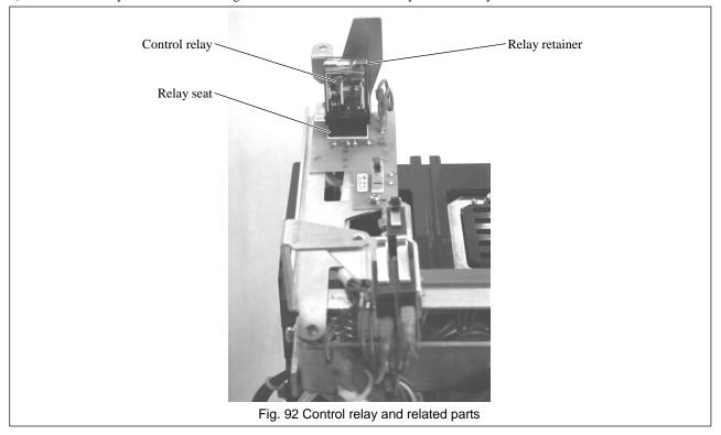
10) Reinstall each part or component in reverse order of removal after inspection. Do not forget to install the OCR ground terminal and the relay base ground terminal.
