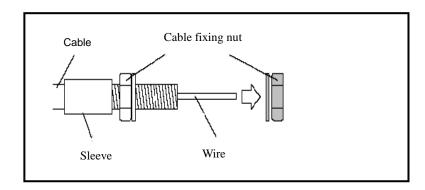
Temporarily tighten the cable fixing nut.
