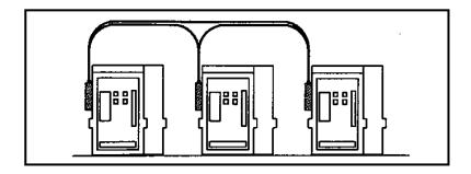
The mechanical interlock system allows up to three ACBs to be selectively turned on or off to the configured requirement.
