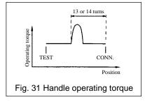
Turning the draw-out handle will unlock the release button.
