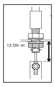
Attach the cable in the cable mounting
