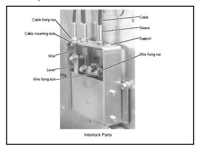
1 Loosen the cable fixing nut and the wire fixing nut.
