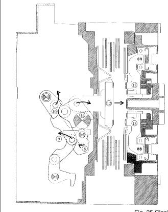
Closing cam ® rotating clockwise causes closing link and top link ⑨ to be pushed straight. This rotates closing toggle cam ⑩ connected with closing link ⑨ counterclockwise, so that crossbar ⑪ rotates clockwise and thus moving contact ⑫ comes in contact with stationary contact ⑬. At this time, each component is positioned as shown in Fig. 27.
