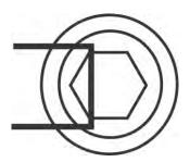
When the handle shutter is at the left of the hole, remove the adjustment plate. This will push against the handle shutter less moving it towards the centre of the hole.
