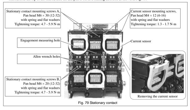
3) Unscrew stationary contact mounting screws A and B.
