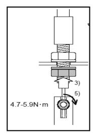
Holding the wire, tighten the
