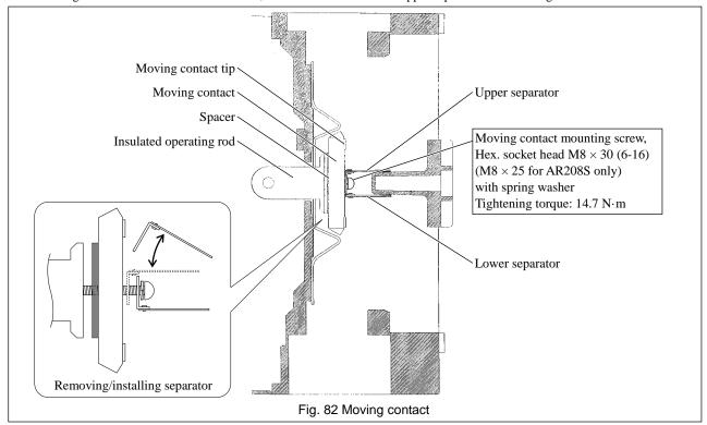
4) Supporting the spacers (the number of which varies depending on the poles), the moving contact, the lower separator, and the moving contact mounting screws by hand, turn the moving contact mounting screws additional two or three turns to remove these parts. Fig. 83 shows the moving contact-related parts.
