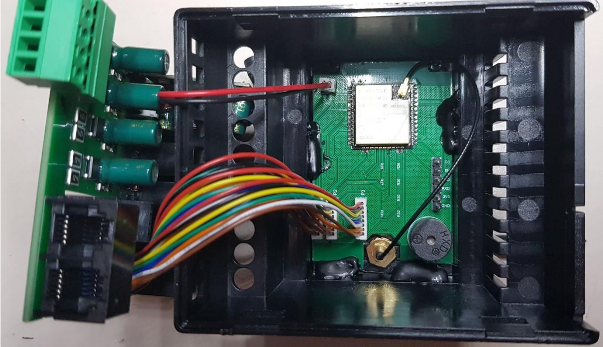
Processor and LED PCB glued in top of case:
