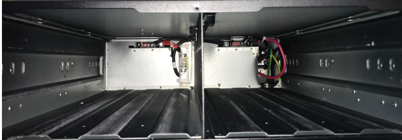
Figure 43: Empty EBM chassis, battery connectors are at the back
