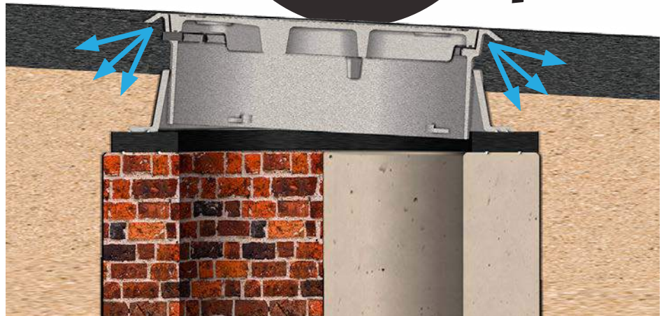
The SELFLEVEL sits on the road surfaces instead of the brick or concrete structure. This allows shock from the traffic to be transmitted to the sub-surface rather than the manhole itself.
