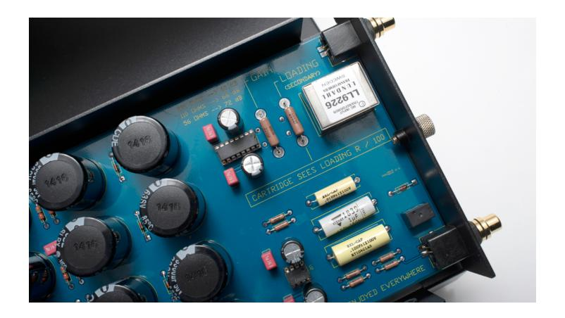
The question of how to offer loading and gain options is a tricky one. All solutions have advantages and compromises. For the *MCX* I decided on the most simplified signal path — along with flexibility in values — as the highest priority.
