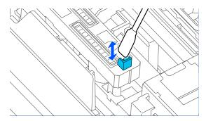
(4) If there is any fluff or dust in the caps, remove it with the tip of the cleaning stick or with tweezers.
