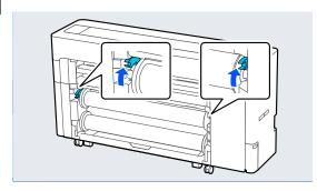
Remove the spindle.
