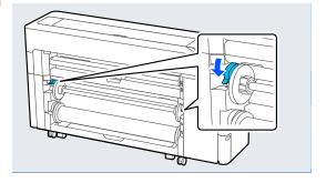
Press the pause/resume button, and then use the take-up direction switch to select either printed side in or printed side out.
