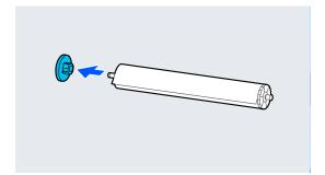
Remove the roll paper from the spindle.
