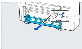
Remove the spindle.
