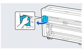
Loosen the screw that secures the cutter with the cross-head screwdriver.
