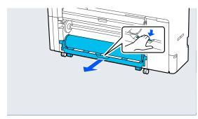
Remove the spindle.
