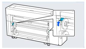
Remove the spindle.
