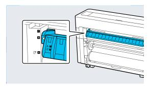
Raise the spindle lock lever for roll1.
