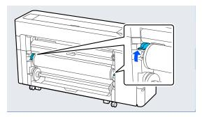
Remove the spindle.
