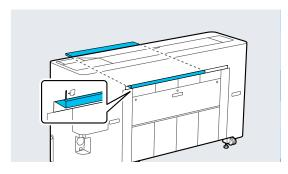
When loading poster board with a paper length of 600 mm or more, pull out the paper basket to reduce bending of the poster board while printing.
