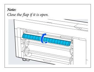
Go to the rear of the printer, align the paper with the alignment position on the left side with the side to be printed facing up.
