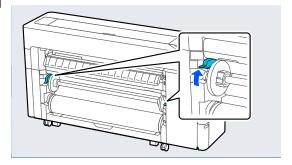
9 Remove the spindle.
