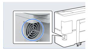
If the printer is particularly dirty, dampen the cloth with water containing a small amount of neutral detergent, and then firmly wring the cloth dry before using it to wipe the printer's surface. Next, use a dry cloth to wipe away any remaining moisture.
