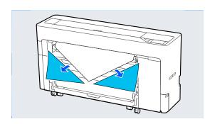
Check the take-up direction and attach the end of the paper to the roll core.
