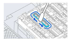
(4) Wipe the edges of all of the capping stations with the flat surface of the cleaning stick.
