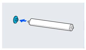
Remove the roll paper from the spindle.
