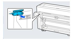
7 Tighten the screw that secures the cutter with the cross-head screwdriver.
