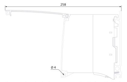
Figure A-2 Dimension drawing CPU 1517-3 PN/DP, side view with open front panel
