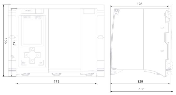
Figure A-1 Dimension drawing of CPU 1517-3 PN/DP, front and side views
