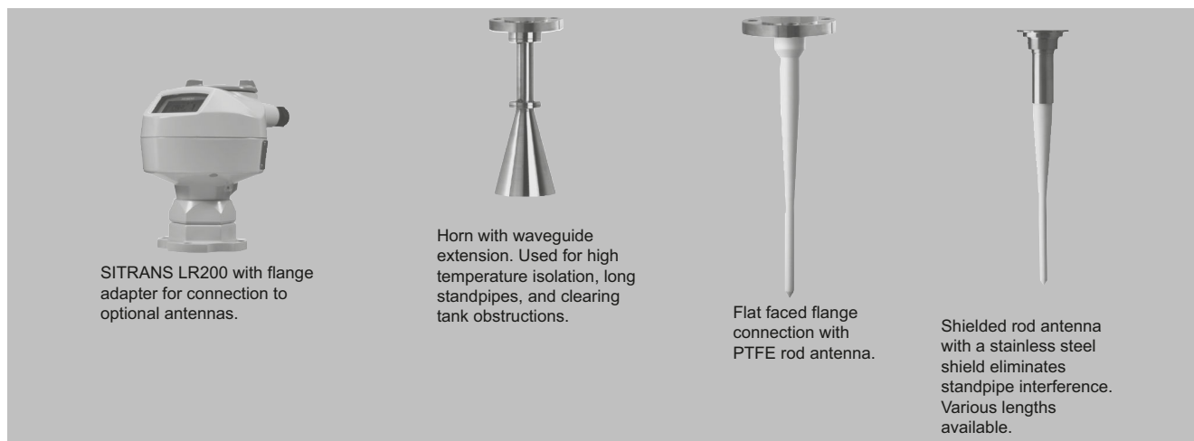
Antenna configurations for SITRANS LR200
