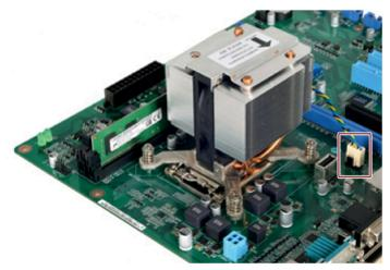
3. Remove the highlighted screws.
