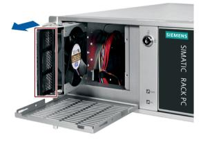
5. Remove the filter in the direction of the arrow.
