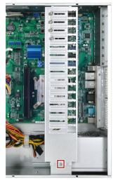
2. Remove the slot bracket of the slot for the expansion card.
