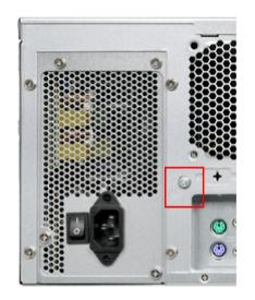
Connect the identified function earth connection to the protective conductor of the control cabinet in which the device is installed.
