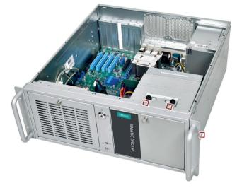
5. Lift the drive cage completely out of the device.
