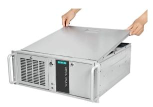
3. Lift the cover from the back and remove it.
