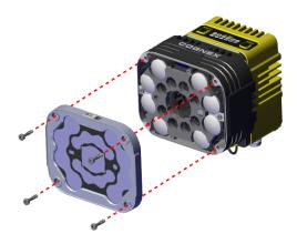
5. Insert the bandpass filter into the sensor.
