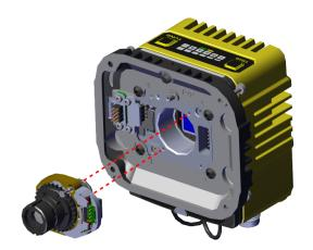
3. Attach the front of the adapter to the sensor.
