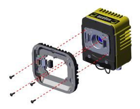
2. Insert the lens and tighten the two captive screws.
