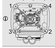
4. Remove the front cover of the adapter.
