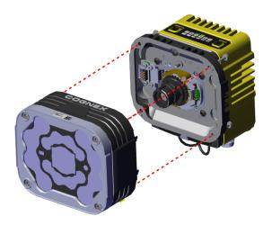
2. Unscrew the two captive screws holding the lens.
