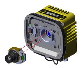
**Note**: When swapping the lens out, make sure not to pull on the lens itself but on the housing of the lens.
