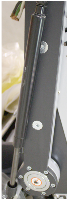
2) Gas Spring (located on swing weight level arms)
