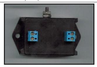
Fire Alarm Class A is 2 Pair, Class B is 1 Pair FA 12VA 12V"A" Zone Protector 2 Pair 12V"B" Zone Protector 1 Pair FA 12V B 24V"A" Zone Protector 2 Pair FA30VA FA30VB 24V"B" Zone Protector - 1 Pair FA30VB-BH 24V+3 amps "BH" Bells Horns 1Pair 34.8V+"B" Zone Protector 1 Pair FA60VB 34.8V+ 3amps "B-NC" Bells Horns FA60VB-NC
