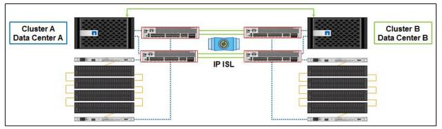
In a two-node configuration, for each (single-node) cluster, the standard cluster interconnects are not required. The hardware requirements for a two-node configuration are different for stretch and fabric implementations.
