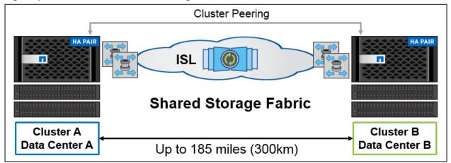
Figure 1) Basic MetroCluster four-node configuration.
