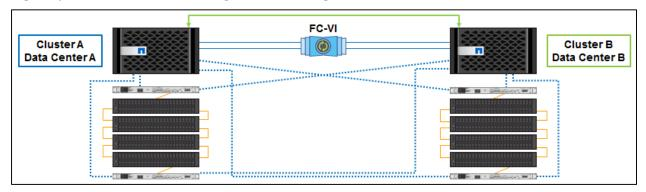
Figure 6) MetroCluster two-node bridge-attached configuration.
