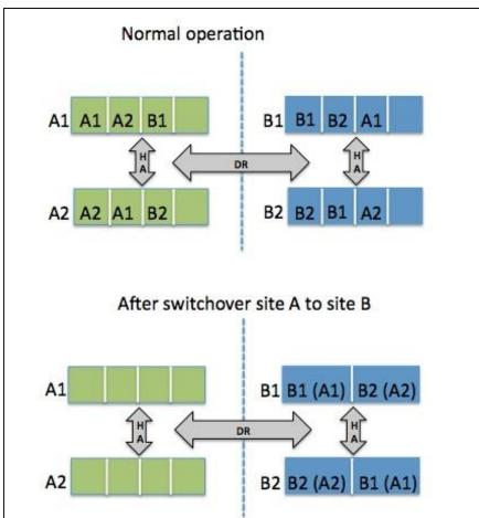
Figure 9) NVRAM segment assignment before and after switchover.
