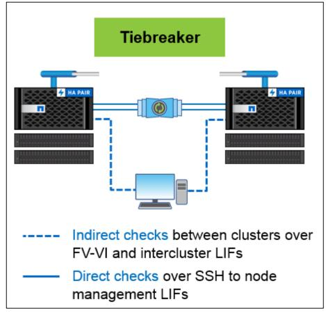
Figure 18) MetroCluster Tiebreaker software operation.
