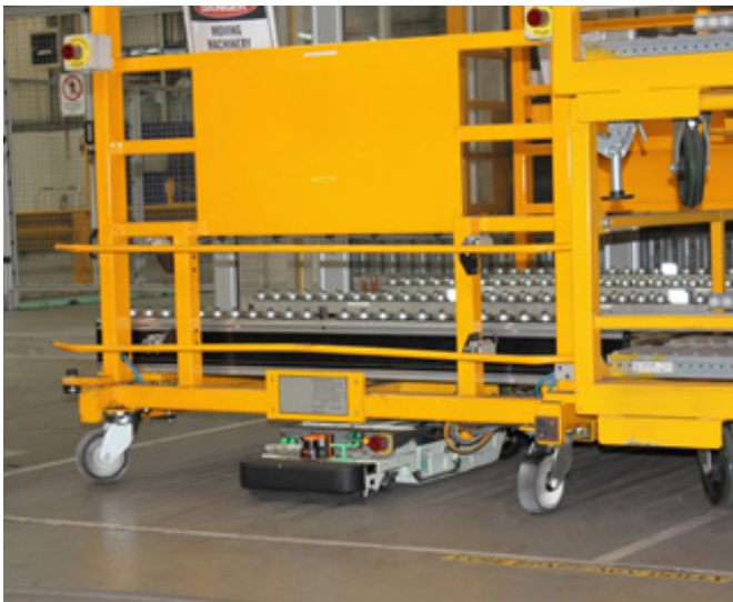
THE PURPOSE OF THE SELF-ALIGNMENT FUNCTION IS TO ELIMINATE FREE SPINNING OF THE SWIVEL CASTOR. THE SPRINGS WILL RETURN THE CASTOR BACK TO DEFAULT FORWARD POSITION.
