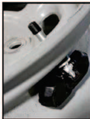
Valve Options for 0.453", 0.625", and 7.7mm Rim Holes
