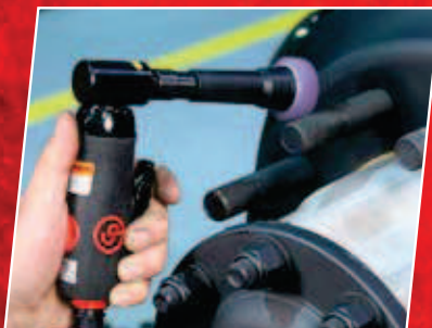
Clean the drum and studs with a CP7562 Mini Angle Grinder
