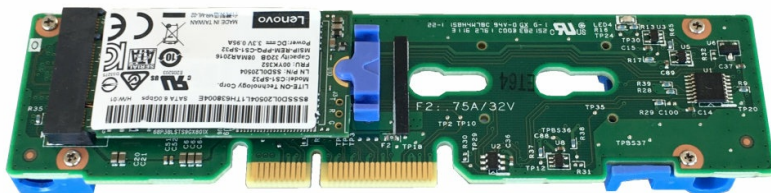
Figure 13. Single M.2 Boot Adapter and a 32 GB M.2 drive
