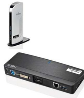
**The main difference** between these is that product-specific Port Replicators (picture A) only grind through the connected notebook performance, while USB Port Replicators (picture B) generate their own system independent performance which extends the overall workplace performance to a certain defined standard (e.g. two times Full-HD - monitor performance).
