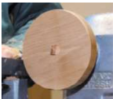
The shelf is wedged on to Martin's jam chuck and can now be trued up
