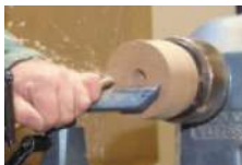
Making the jam chuck
