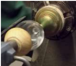
The parts are glued together and allowed to dry between centres
