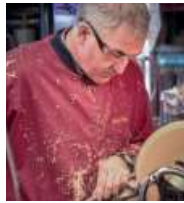
A glued segment ring is mounted on the Cole jaws for cleaning up
