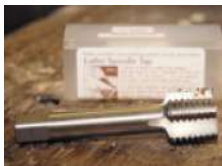
This tap matches the lathe spindle thread
