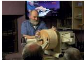
Another large glued set of rings are mounted on the lathe with an MDF plate on the tailstock
