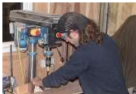
Drilling the walnut blanks for the clamp
