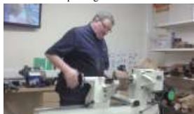
Emmet Kane mounts a burr for turning
