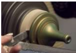
The waxed foot ready to be parted off
