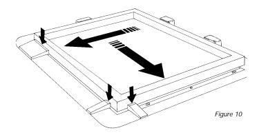
Adjustable master frames are equipped with push pins that adjust in half inch (1/2") increments to fit a variety of frames. Remember, frame width dictates image centerline. To adjust push pin, push locking cam to unlock position Adjust push pin barrel to the desired position and push locking cam back to the locked position. (See Fig. 11)
