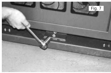
4. Additional leveling adjustments are made by alternately adjusting the two rear leveling legs located at the rear bottom of the chassis. (See figure 8 below)
