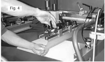
4. Turn the flood pressure knobs clock-wise, to adjust flood bar all the way up. (See Fig. 5)
