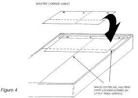
If you are using a fully adjustable exposure frame, your layout table should have 2 center lines, one for the 23" wide frames, and one for the 25" wide frames. When pasting up films to carrier sheets it is important to use the centerline that corresponds with the frame size that will be used for that job. (ie: 23" frame = 11.5" centerline)When pasting up films, the main or "trap color" should be positioned first and taped securely to the pin mounted carrier sheet.(See Fig. 5)
