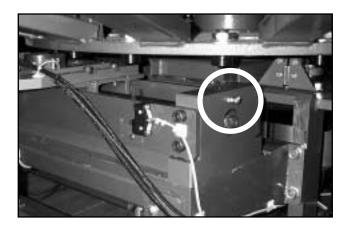
5. Open manual shut-off valve for compressed air supply to the equipment. The manual shut-off valve is open when the handle is aligned with the incoming compressed air supply line pipe or hose. (See illustration at right)
