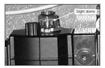
2. Should the oil flow rate require adjustment, use the small standard blade screw driver and adjust the small red colored metering screw on top of the sight dome for the proper rate of 1 drop for every 2 complete press cycles. Turn the metering screw clockwise to decrease the oil flow rate. Turn the metering screw counterclockwise to increase the oil flow rate. (See top view illustration at right)
