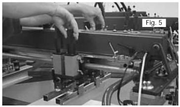
5. Pull the print carriage all the way towards the front of the print head and disconnect the 3/8" air line located on the front of the head (ToI-O-Matic Cylinder Fitting). Use a brass fitting union with plug, to plug the 3/8" air line (M&R Part #2003060-fitting union and Part # 2003042-plug).
