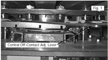
This convenient control lever allows the press Operator to adjust the off-contact setting for the press from a maximum of 3/16" (5mm) to the minimum setting. The adjustment is calibrated in three settings at 1/16" (1.5mm) increments.
