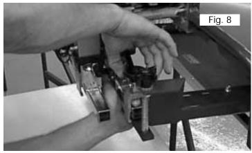
The height of the heat panel may be adjusted by using the black plastic cross knobs, which are threaded onto the threaded support rod on top of the flash panel mounting bracket. (See Fig. 9)
