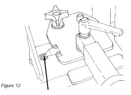
Now you are ready to install the Tri-Loc pallet and mark the press for "Prime Position". Remove one print pallet and replace it with the Tri-Loc pallet. When installed, the M&R logo should be facing the operator and the registration stop blocks will be on the left side.
