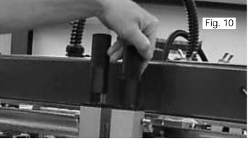
9. Bring pallet down by pressing the green reset button, now use your small magnetic level (Torpedo Level) and place it on the edge of the flood bar to make sure it is level. If it is not level, make the necessary adjustments to make it level. (See Fig 11)
