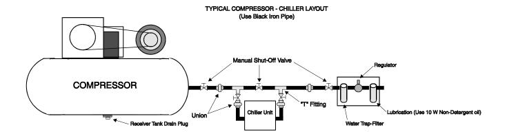
Figure 1 Typical Compressor-Chiller Layout
