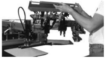
Now pull "OUT" the small knurled knob located at the upper right side of the "Flip Up Front Screen Frame Holder" assembly. This will release the locking pin mechanism, allowing the front screen frame holder assembly to swing down into normal print position. Locate the "U" shaped locking bracket into the lock mechanism and pull up on the red locking lever to secure the front frame holder assembly back in place. (See top left next page)
