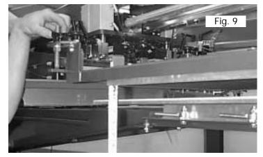
8. To adjust the infrared panel at the rear for proper level, adjust the black plastic cross knob located at the rearunistrut support channel under the infrared panels insulated cover guard. (See Fig. 9A top right)
