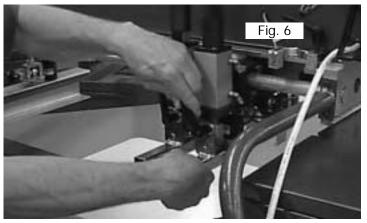
6. Next, adjust the squeegee/flood bar pressure adjustment knobs (turn clockwise) until the squeegee/flood bar is fully raised. In this position the squeegee/flood bar will not perform the "chopper" motion in the event the print station is inadvertently turned on. In this way damage to the radiant panel is eliminated. (See Fig. 7 top left next page)
