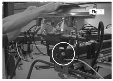
Adjust both the squeegee and flood bar height adjustments to the full up position to maximize the clearance between the Quartz Flash unit and the print carriage assembly. Additionally, adjust both the flood and squeegee speed controls to their minimum settings. (See figure 2 below)
