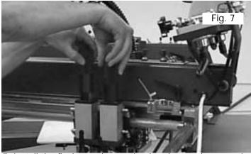
7. Install the flash panel mounting bracket on the mounting bar and secure with two squeegee clamps (manual) (See Fig. 8)
