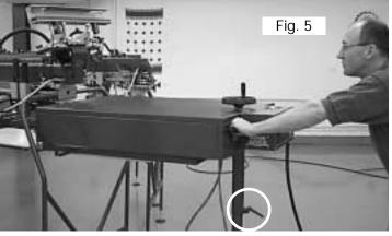
5. Check to be sure the front mounting bar is straight (no angle) by loosening the two ratchet knobs (Kipp Elisa Knobs) and turning the mounting bar. (See Fig. 6)
