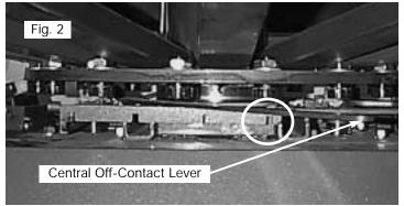
When the lever is all the way towards the left hand side, which is the lowest position of the table, this gives you the most off-contact setting, which is 3/16" (5mm) added to your initial off-contact. (See Fig. 3)
