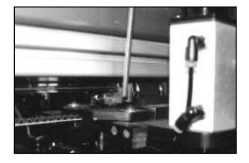
6. Adjust the 1/4"-20 X 1-1/4" allen head cap screw in a clockwise direction to increase the tension on the timing belt. Generally, this will only be a slight adjustment, perhaps 1/4 to 1/2 turn of the screw. (See illustration at right)
