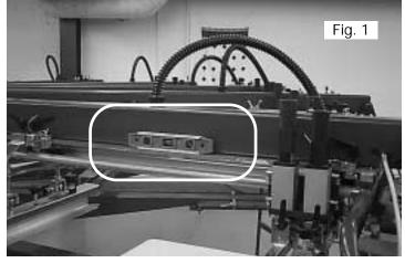
Adjust the leveling pads on the head support to level the head if necessary. (See Fig. 2)
