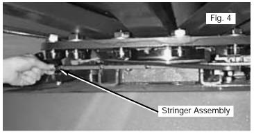
Each setting is designed to change the off-contact setting by 1/16" (1.5mm).
