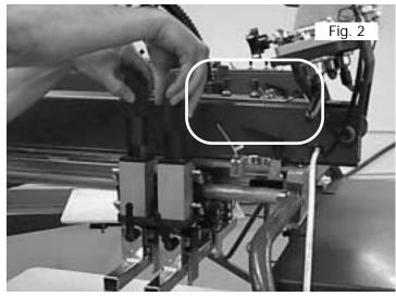
The M&R Quartz Flash unit will produce excellent cure results when properly leveled. It is imperative that the heating element assembly be parallel to the pallet surface. The preferred dimension between the surface of the heating elements and the pallet surface is 2-1/4" as measured at all four corners when the index carousel is fully raised. (See figure 3 above right)
