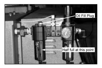
5. To add oil, use the standard blade screw driver to remove the fill plug at the top of the lubricator assembly. Add 10 wt. non-detergent oil (M&R Part No. 7017000) as needed to bring oil to proper level. The glass indicator will indicate full when the oil level is approximately 1/8" from the top of the glass indicator. Replace the oil fill plug and tighten securely. **NEVER OVERFILL THE LUBRICATOR RESERVOIR!**
