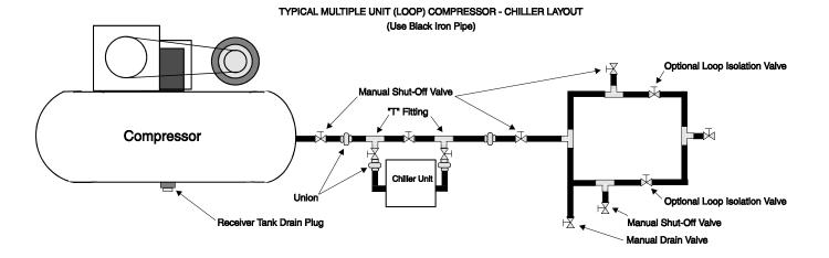
Figure 2 Typical Multiple Unit (Loop) Compressor-Chiller Layout
