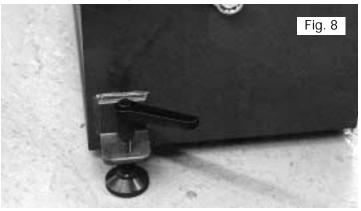
5. When leveling adjustments are completed, tighten the 3/4" pivot hex head bolts and the rear leveling leg adjustments.
