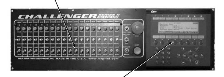
**E300 Operator Interface Instructions:** The Operator Interface control panel incorporates an L.C.D. (Liquid Crystal Diode) type alpha/numeric display for providing information regarding operational, programming and system status messages in real time. Refer to page 41 of this Manual for a detailed description of the operation and function of this control.
