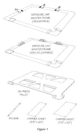
To better facilitate shops that have existing film/pin systems, the M&R Tri-Loc is offered without a film register Pin Bar attached. Pin Bars and carrier sheets are available separately or in a start up kit available through M&R Sales and Service. It is important to note that the greatest factor affecting quick set ups and on press registration, is properly separated films that have been accurately registered to one another using some type of "Pin Bar" system.
