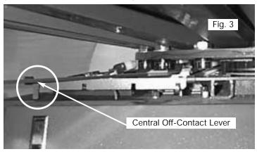
In order to adjust the lever, the index table should be in the lowered position. Taking your left hand and lifting up on the stringer, you can now manually move the lever to the desired position for the off-contact setting. (See Fig. 4)
