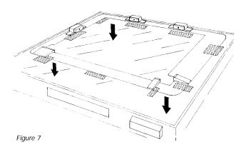
The majority should be used under the working fixtures. (ie: Stop blocks and push pins). Thoroughly clean the master frame and glass for proper tape adhesion. Position master frame on the exposure unit leaving proper clearances and mark the outer edges with masking tape for a reference. (See Fig. 6)
