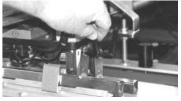
Adjust the flood bar pressure by use of the large black knurled knobs at the top of the print carriage assembly. The flood bar pressure should be adjusted so that there is only a slight pressure felt on the bottom of the screen mesh. To increase the flood bar pressure, turn the black knurled knobs counterclockwise. To decrease the pressure, turn the black knurled knobs clockwise. With the flood bar installed, you are now ready to install the squeegees.
