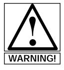
WARNING! THE NEW BATTERY MUST BE INSTALLED WITH IN FIVE (5) MINUTES OF REMOVAL OF THE OLD BATTERY. THIS WILL ENSURE THE PRESERVATION OF DATA IN THE SERVO AMPLIFIER MEMORY.
