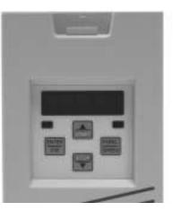
The L.E.D. display automatically changes to display either flood stroke or squeegee speed as the print station operates through the flood/print cycle.
