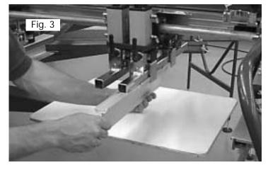
3. Adjust the flood bar for zero angle . Loosen the two ratchet type knobs on both sides of the mounting bar. After adjusting, tighten the knobs. (See Fig. 4)
