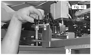
10. Set the inboard speed and the outboard speed of the infrared panel by adjusting the squeegee and flood bar speed controls located on the top of the print station. (See Fig. 11)
