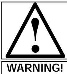
**WARNING! THE NEW BATTERY MUST BE INSTALLED WITH IN FIVE (5) MINUTES OF REMOVAL OF THE OLD BATTERY. THIS WILL ENSURE THE PRESERVATION OF DATA IN THE PLC MEMORY.**
