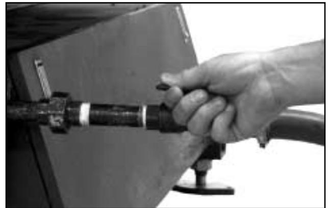
3. Bleed off any compressed air which may remain in the system by opening the small pet-cock valve (turn handle counterclockwise to open valve) at the bottom of the moisture trap assembly. Allow any compressed air to completely evacuate the system, the needle on the air gauge should read zero, before closing (turn handle clockwise to close) the pet-cock valve.
