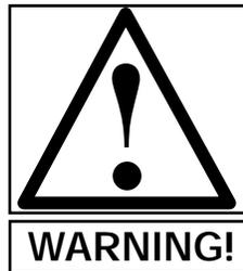
**WARNING!** The electrical power switch for the Challenger Series II must NOT be turned "OFF" before the flash cure panel has cooled down to at least 99 degrees or lower.
