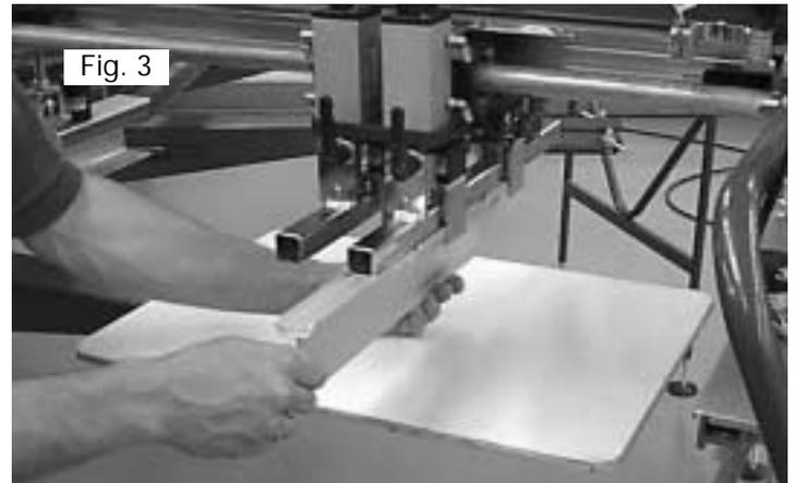
3. Adjust the flood bar for zero angle. Loosen the two ratchet type knobs on both sides of the mounting bar. After adjusting, tighten the knobs. (See Fig. 4)
