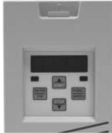
The L.E.D. display automatically changes to display either flood stroke or squeegee speed as the print station operates through the flood/print cycle.
