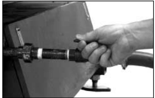
3. Bleed off any compressed air which may remain in the system by opening the small pet-cock valve (turn handle counterclockwise to open valve) at the bottom of the moisture trap assembly. Allow any compressed air to completely evacuate the system before closing (turn handle clockwise to close) the pet-cock valve.
