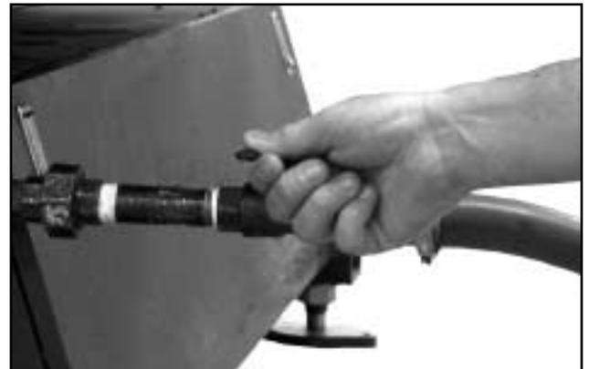
**NOTE: The manual shut-off valve is not supplied with the equipment. The manual shut-off valve must be installed by the end user.**
