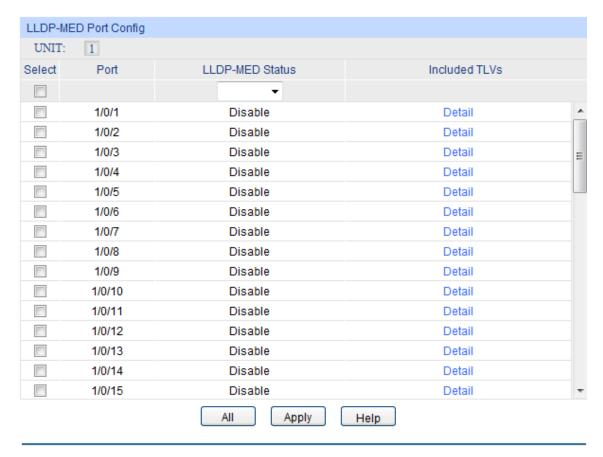
Figure 15-7 LLDP-MED Port Configuration
