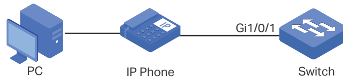
Figure 6-1 LLDP-MED Network Topology
