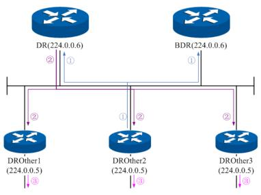
Figure 10-33 Flooding of the LSA
