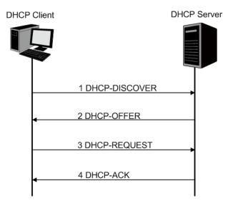
Figure 10-7 The Process of DHCP
