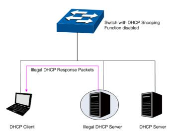
Figure 14-7 DHCP Cheating Attack Implementation Procedure
