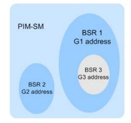
Figure 11-19 BSR Domain Divided by Multicast Address
