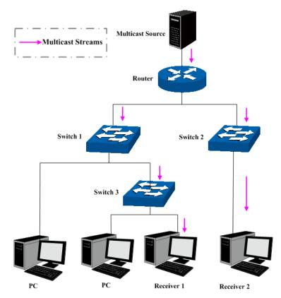
Figure 9-1 Information transmission in the multicast mode
