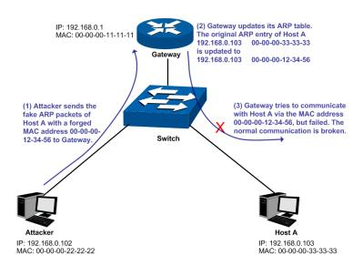
Figure 14-11 ARP Attack – Cheating Gateway
