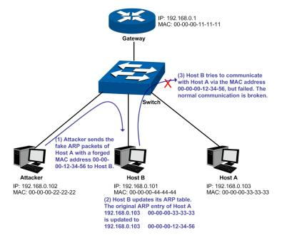
Figure 14-12 ARP Attack – Cheating Terminal Hosts
