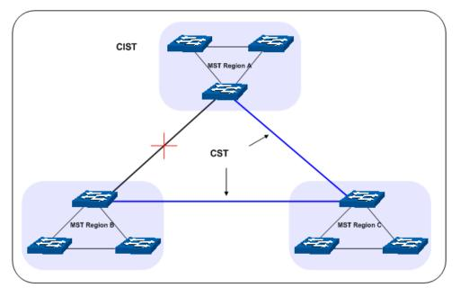
The following figure shows the network diagram in MSTP.
