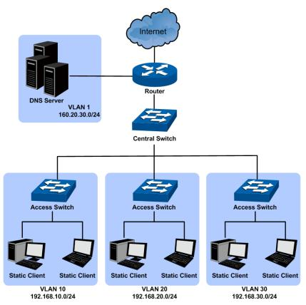
Use T3700G-52TQ as the central switch and enable its DHCP server function to allocate IP addresses to clients in the network. Enable the DHCP relay function on each access switch in VLAN 10, 20 and 30. For details about DHCP relay, please refer to <u>10.5 DHCP Relay</u>.
