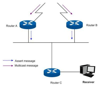
Figure 11-12 Assert Mechanism
