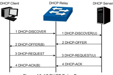
Figure 10-17 DHCP Relay Process
