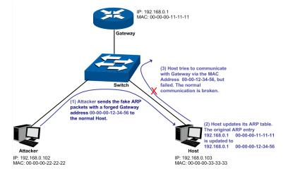
Figure 14-10 ARP Attack - Imitating Gateway
