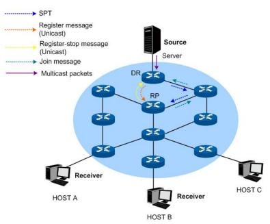
Figure 11-18 Multicast Source Register Topology in PIM SM
