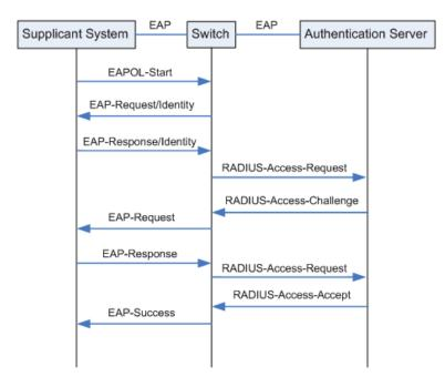
Figure 14-20 EAP-MD5 Authentication Procedure
