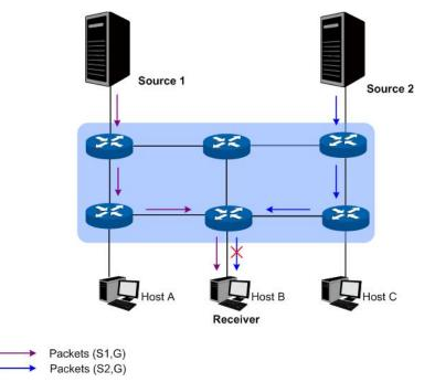
Figure 11-4 IGMPv3 Multicast Source Filtering
