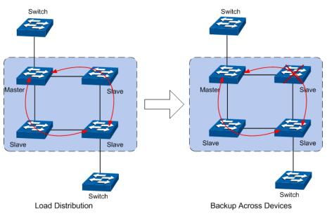
Figure 5-2 Load Distribution and Backup across Devices
