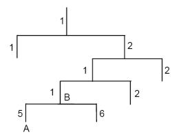
Figure 15-2 Architecture of the MIB tree
