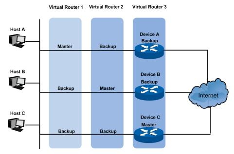
Figure 10-58 VRRP Load Balancing
