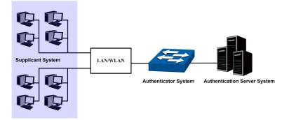
Figure 14-19 Architecture of 802.1X authentication
