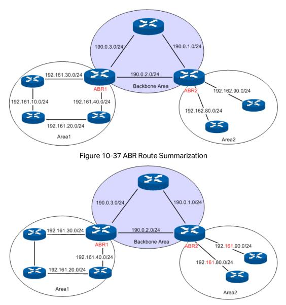
Figure 10-38 Discontinuous Network Segment
