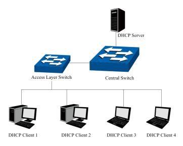
Figure 14-5 Network diagram for DHCP-snooping implementation
