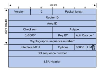
Figure 10-41 DD Packet
