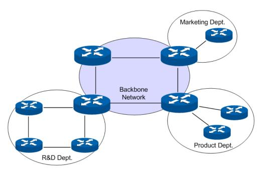
Figure 10-30 Common Scenario for OSPF routing protocol
