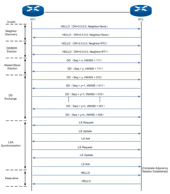
Figure 10-32 Steps to Establish a Complete Adjacency Relation
