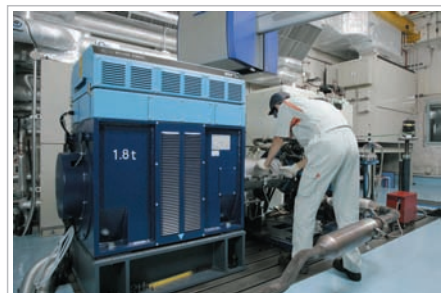
Oil pump test on engine dynamometer
