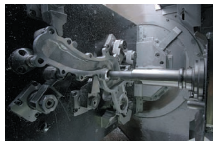
High precision machining process for Water Pumps
