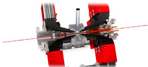
Figure 1. A sectional view of the PolarX-EBIT. The photon beam is overlapped with the prolate ion cloud in the center.
