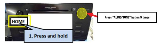
• Switch the unit into "Diagnosis Mode" by pressing and holding the HOME button while pressing the "AUDIO/TUNE" button 5 (five) times.
