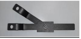
**Engine support cross member** (900030490): This tool is used together with tool 900029751 to support the engine after the gearbox has been removed.
