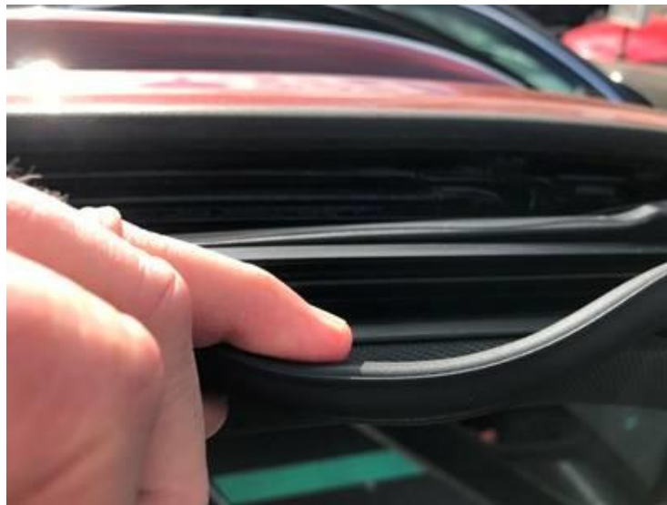
Figure 3. Partial removal of sunroof's inner seal.
