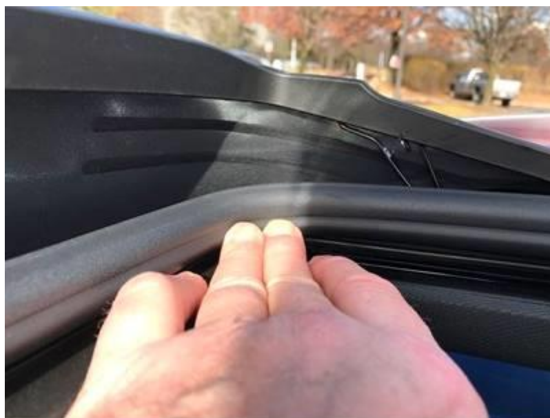
Figure 7. Sunroof inner seal pressed back into position.
