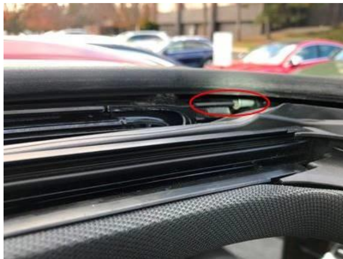
Figure 2. Sunroof drive cable entry.
