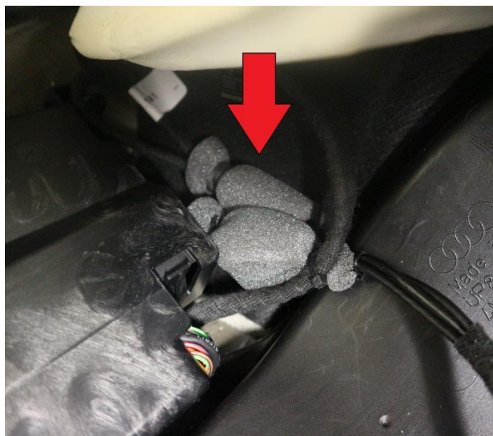
Then move the cable out of the way, positioning it to the side of the gateway ECU support.
