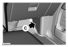
The third interior set (C) is taped on a wire harness by the passenger side footwell. This set is the other end of the circuits taped under the hood at the powertrain control module connector. Remove the fuse panel access door in the kick panel to access the wires. If you do not see them, you may need to pull them down.
