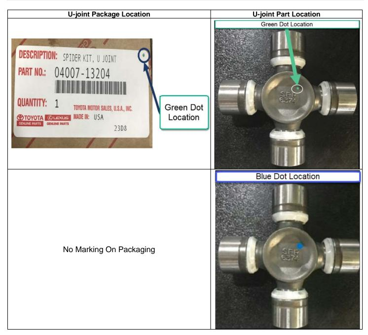
NOTE: The U-joint package and the U-joint should both have green dot; if both do not have a green dot, the part SHOULD NOT be used.
