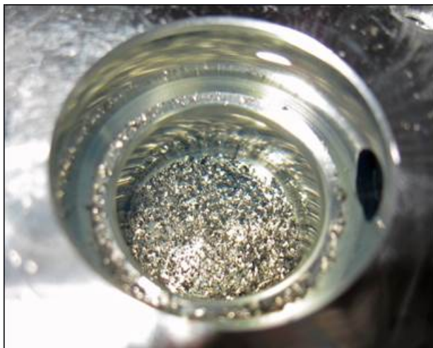
Figure 6. Valve Bore with Metal Particles
