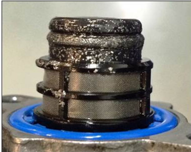
Figure 5. N290 Fuel Metering Valve with Metal Particles
