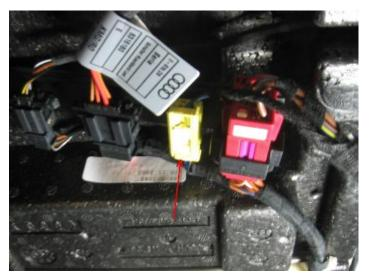
**Figure 1.** The yellow airbag connector located below the rear seats.
