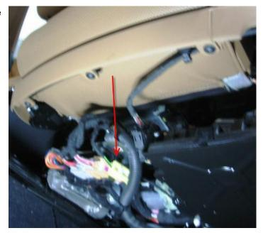
**Figure 2.** The yellow airbag connector located beneath the front seats.
