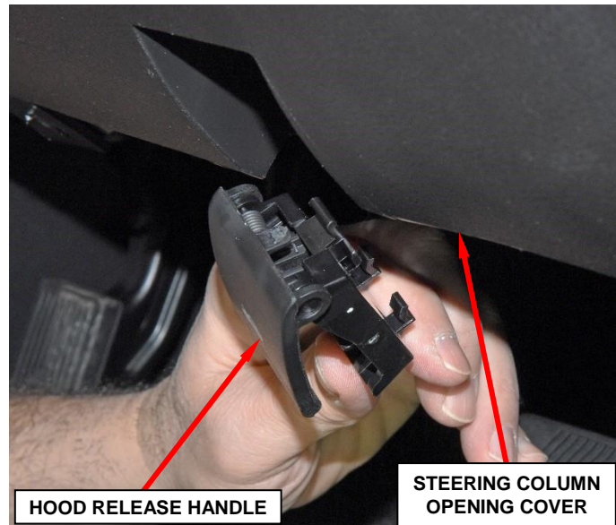
Figure 2 – Hood Release Handle
