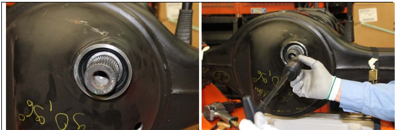
Figure 5 – Thru-shaft Oil Seal Removal
