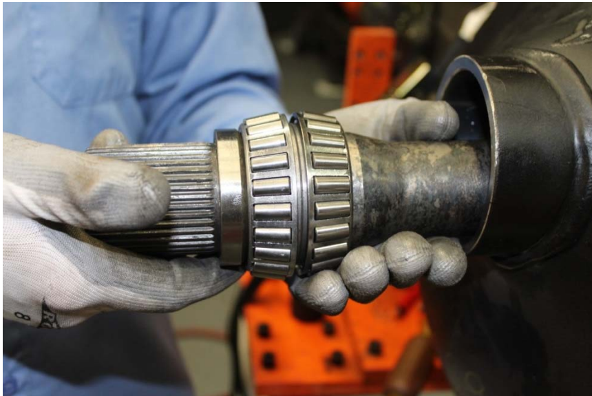
Figure 9 – Thru-shaft and Bearing Assembly Installation
