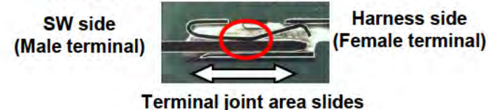
Head light terminal is melted
