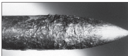
Mechanically cleaned point of a pulled-out DX fastener
