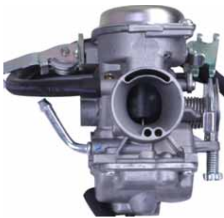
14-CB165-28 28mm YBR125 CV Type (Diaphragm type)
