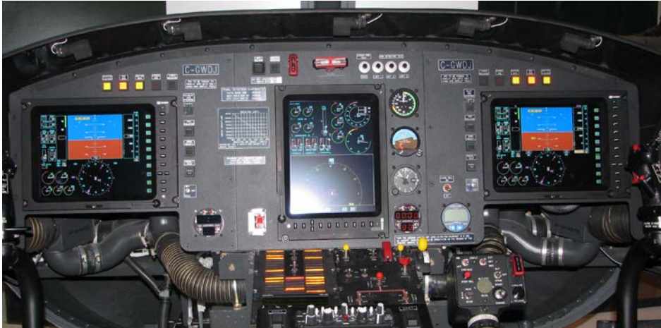
SAGEM Three (3) Display Electronic Flight Instrument System with AHRS System
