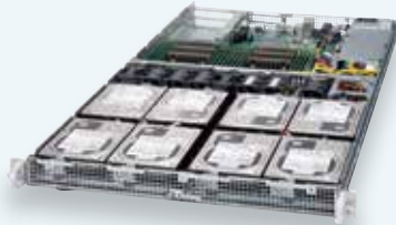
SYS-6018R-TD8 Supports 8x 3.5" & 2x 2.5" Fixed SATA3 Drive Bays
