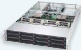
SYS-6028U- TNR(4T/T)+ SYS-6028U- TR(4/4T/T/TP)+ Titanium Level (96%+) Power Up to 4 NVMe Support
