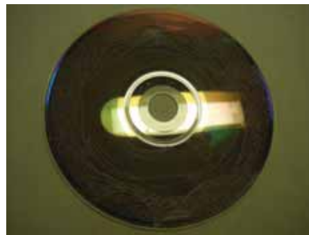
Fig. 4. Image of buckling after deposition of 3 μm-thick AlO x N y dielectric layer.
