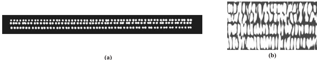
Fig. 2. Results of sub-Bragg and sub-Nyquist holographic search. (a) 180 auto-correlation peaks from sub-Bragg 2D multiplexing. (b) Part of 600 auto-correlation peaks from sub-Nyquist & sub-Bragg recording.
