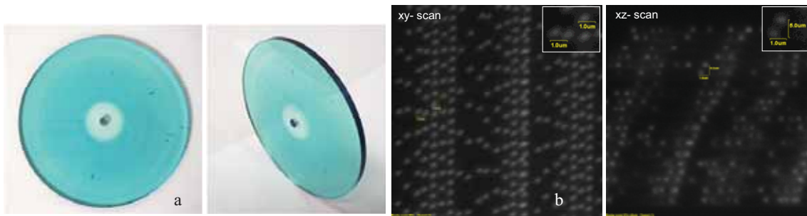
Fig. 3. Photograph of 120mm diameter disk after recording. typical xy confocal microscope scan throughout the different layers and xz confocal microscope scan of \sim 20 layers. Track pitch of 0.8\mu\text{m} and layer spacing of 5\mu\text{m} recorded in the 120mm diameter disk recorded at 7\text{nJ}/\text{bit} from a single pulse of a 75\text{MHz} repetition rate laser.
