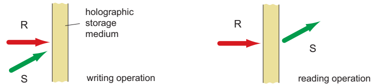
Fig. 1. Conventional holographic recording and read-out process; writing and reading operation are unidirectional.
