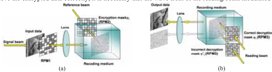
Fig.1 Schematic diagrams of two-wave encryption (a) encryption process, (b) decryption process
