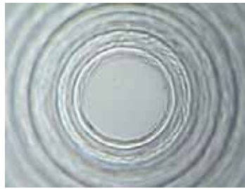
Fig. 5. Micrographic image of the SIL surface after a collision at an approach speed of 0.05 m/s. No scratch was found.
