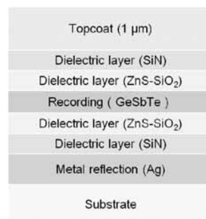
Fig. 1. The medium structure with topcoat layer. Films such as the recording material (GeSbTe), two dielectric layers of \text{Si}_3\text{N}_4 and \text{ZnS-SiO}_2 , and the metal-reflection layer (Ag) were sputtered on a 1.2 mm polycarbonate substrate. The topcoat layer was made by spin-coating.
