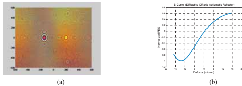
Fig. 5. (a) Diffractive astigmatic reflector with a four level binary surface relief. (b) FES diagram.
