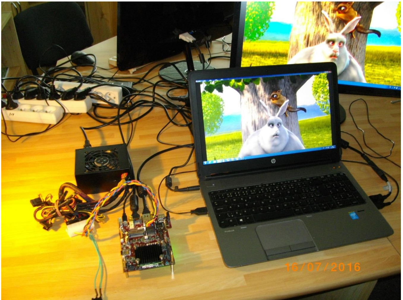
Figure 2: HW accelerated motion detection in Full HD with 60 FPS video processing speed.
